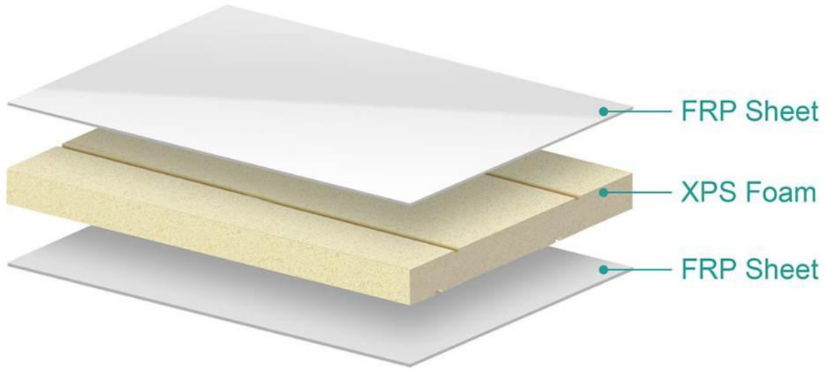
Schematic Diagram of FRP Facing XPS Foam Sandwich Panels
