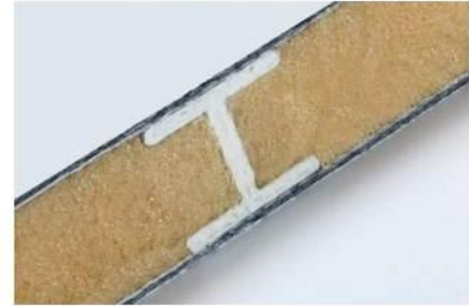
I-shaped Reinforced Structure
